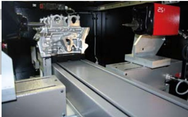
Engine block marking by two i52
