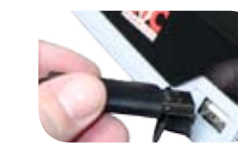
USB connection on the front panel: import/Export of marking files - Keyboard external plug
