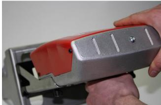
Compromise between robustness and lightness thanks to a cast aluminum body, total weight of 3.7kg
